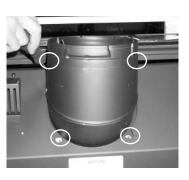
2) Rotate the elbow 180°
